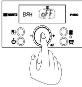
3. Press the 'Dial Button' so 'oFF' is blinking. Then turn the 'Dial Button' clockwise so 'on' is blinking.
