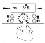
5. Press the 'Dial Button' to store the current setting and return back to 'Installer Mode'.
