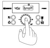
13. Press the 'Dial Button'.'b:noH' will being to flash on the display.
