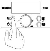
1. Turn off the power to the control panel. Press and hold the 'Function Button' for approximately 5 seconds to get into the 'Installer Mode'.
