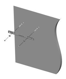
5. Lift up the Combi Boiler, rest the unit on the hooks provided on the wall bracket that is already mounted on the wall.
