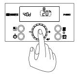
17. Press the 'Dial Button'. The default design cold weather temperature (20°F) will flash on the display. Turn the 'Dial Button' to adjust to the desired temperature.
