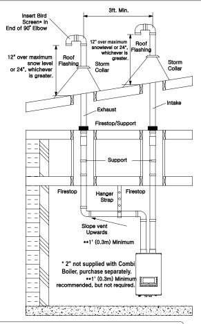
When choosing intake and exhaust terminations, you must use the same type of elbow (i.e. both 90° elbows).
