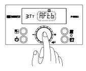
7. With '3:TY' displayed, press the 'Dial Button'. 'A:Ftb' will begin flashing (default). Turn the 'Dial Button' clockwise to select the appropriate heating system type. Press the 'Dial Button' to confirm the setting.
