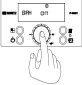
4. Press the 'Dial Button' to save the setting. If you would like to move to next function in the 'Installer Mode', turn the 'Dial Button' clockwise or to exit 'Installer Mode' press the 'Function Button'.
