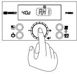
9. With '4:Od' displayed, press the 'Dial Button'. 'A:HI' will begin flashing.
