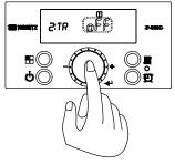
4. Press the 'Dial Button'. OFF will begin blinking. Turn the 'Dial Button' from OFF to ON.
