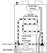
2) When the water filling is finished, then the 3-Way Valve will be switched to heating supply pipe and proceed to add water to increase the pressure on the heating loop.
