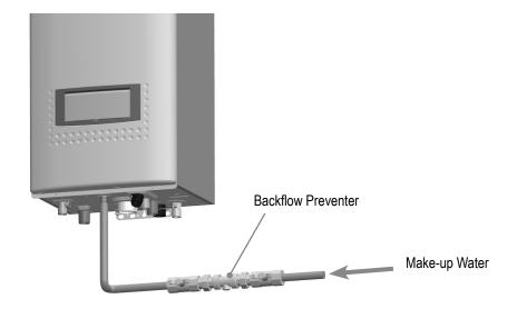
• External water feeder may be installed on the system piping if it is required for specific applications. See the following figure for an example of external water feeder installation on the system piping.
