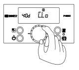
16. Turn the 'Dial Button' until 'C.Lo' is displayed. 'C.Lo' allows for adjustment of the design low temperature setting.
