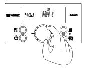
8. Turn the 'Dial Button' until '4:Od' is displayed. '4:Od' allows for adjustment of the design outdoor temperature range.
