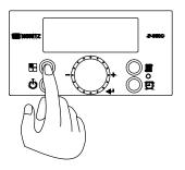
2. Turn off the power to control panel. Press and hold the 'Function Button' for approximately 5 seconds to enter the 'Installer Mode'.
