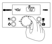
10. Press the 'Dial Button'. The default design warm weather temperature (70°F) will flash on the display. Turn the 'Dial Button' to adjust to the desired temperature.
