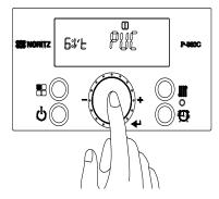
Press the 'Dial Button' ('PVC' will be blinking), then turn the 'Dial Button' clockwise so 'CPVC' is blinking.
