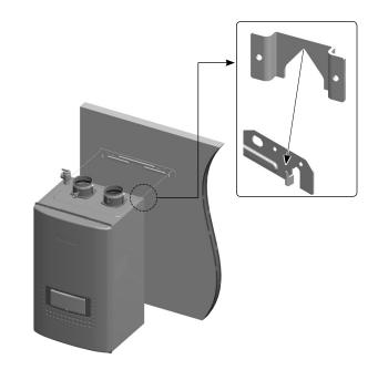
6. Locate the lower mounting bracket on the bottom of the Combi Boiler. The two screws and dry wall anchors will be used to securer the bottom of the unit to the wall.
