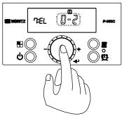
3. '0-2' will flash when the 'Dial Button' is pressed. (The default setting is '0-2' for installations at 0~1,999ft elevation.)
