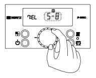
4. Turn the 'Dial Button' clockwise to select the value that corresponds to the installation elevation.
