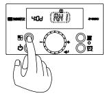
19. To return to the 'Installer Mode' main menu, press the 'Function Button'. Use the 'Dial Button' to scroll through the other menu options.
