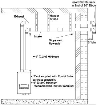
When choosing intake and exhaust terminations, you must use the same type of elbow (i.e. both 90° elbows).
